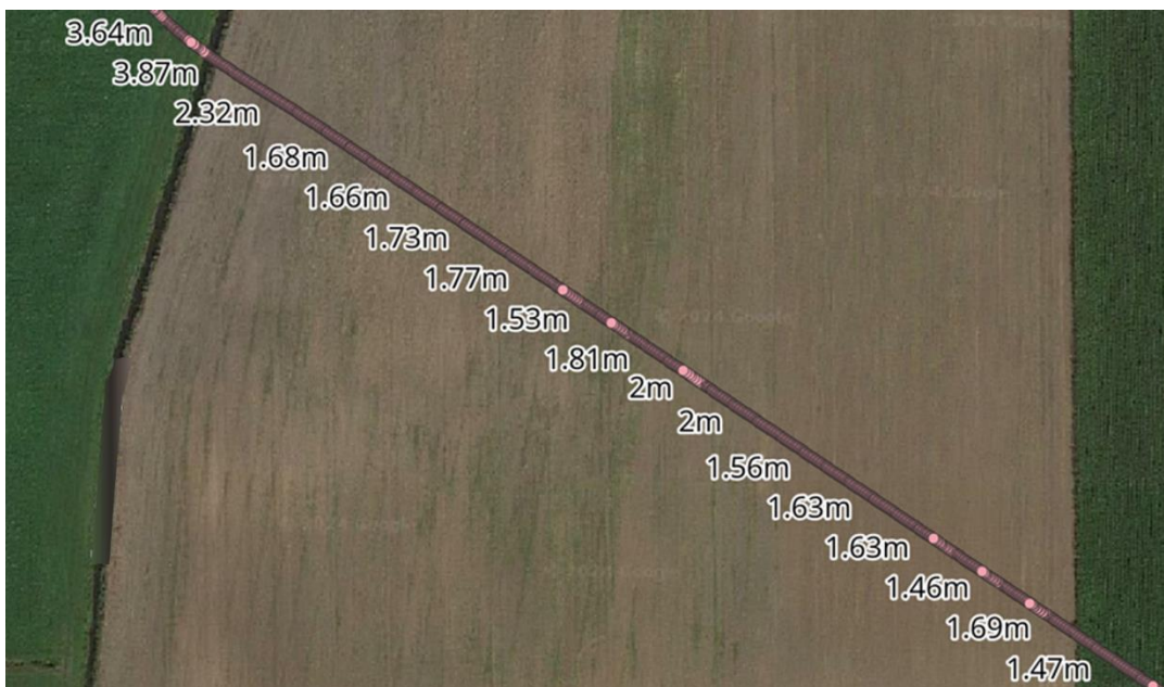
Figure 9 : XY position and DOC as measured along a section of the entire pipeline length
