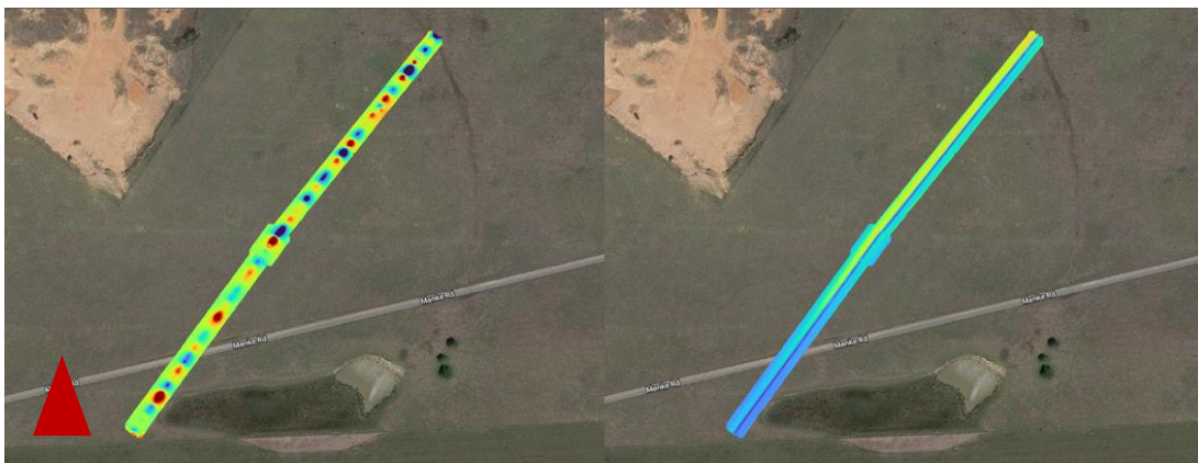
Figure 4: Total magnetic field overlay image of the inspected area: low frequency map (left) high frequency map (right).
