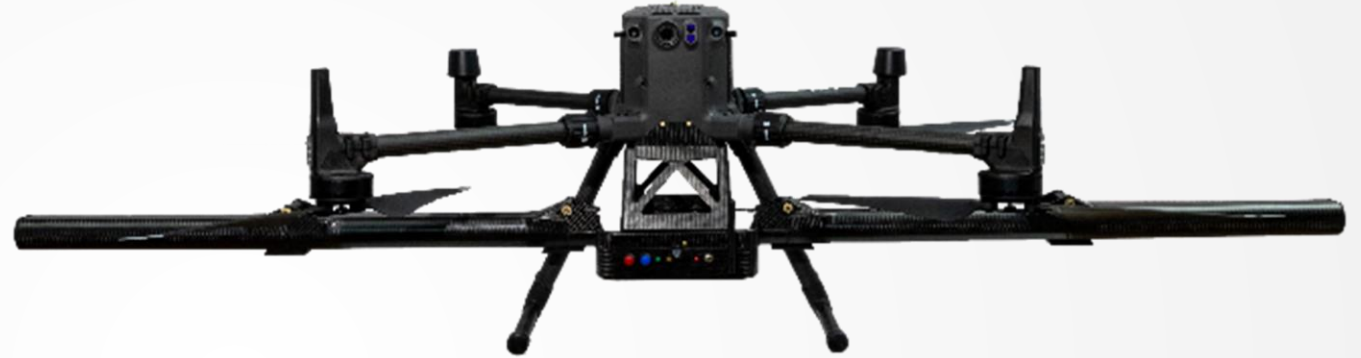
Skipper NDT's embedded system mounted under an off-the-shelf UAS
