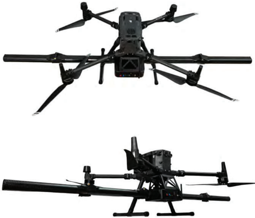
Figure 1: The embedded system, mounted on an off-the-shelf UAS (DJI M300).
