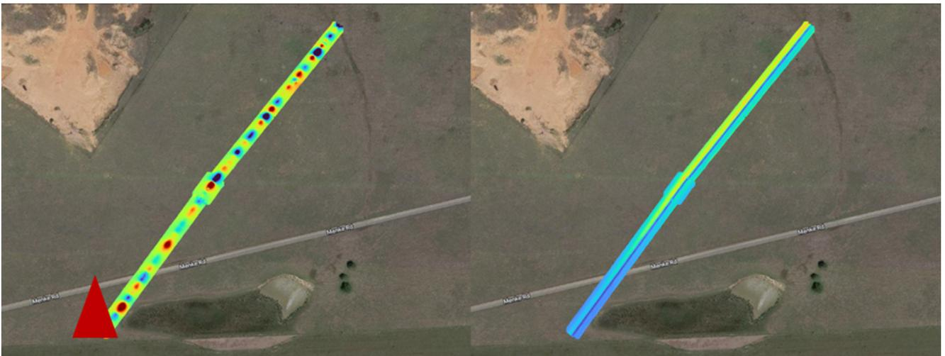
**Figure 5:** Total magnetic field overlay image of the inspected area: low frequency map (left) high frequency map (right).
