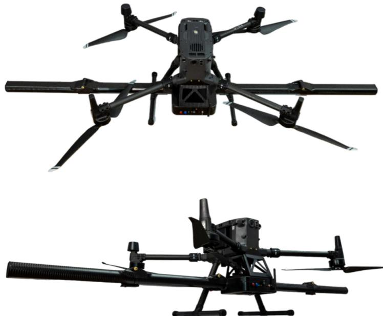
**Figure 1:** The embedded system, mounted on an off-the-shelf UAS (M300).
