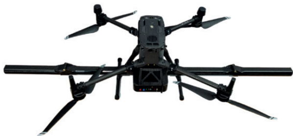
Figure 1. The Skipper NDT Embedded System mounted on an off-the-shelf UAS (DJI M300).
