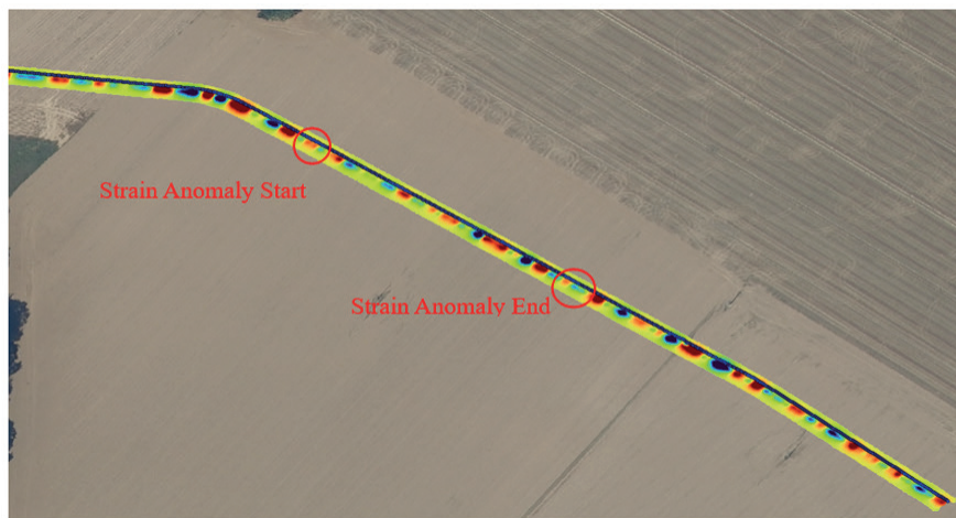
Figure 5. Bending strain plots (top) showing vertical anomaly and magnetic map variation (bottom).
