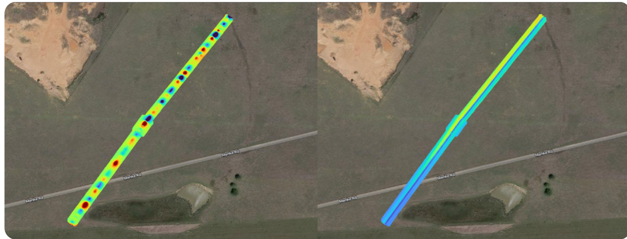
Figure 4 : Total magnetic field overlay image of the inspected area (high frequency map)
