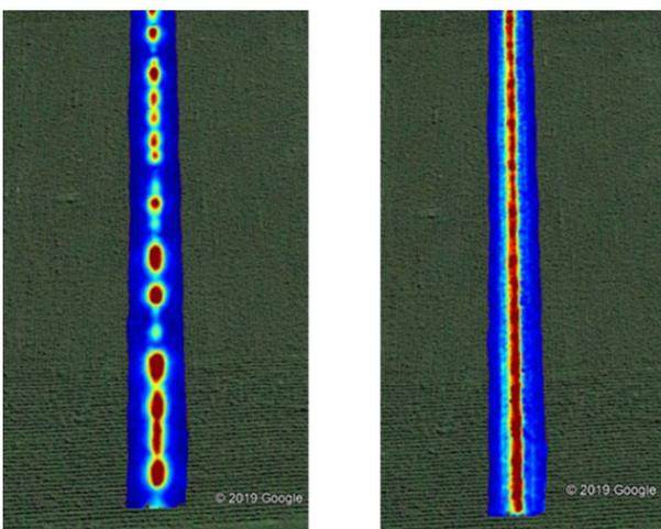
Figure 3. Resulting magnetic maps of the previous inspected area. The two maps rely on the same dataset but treated with different algorithms.
