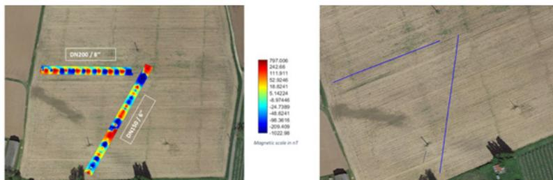
Figure 4. Magnetic maps of each inspected areas with its corresponding colorbar (in nanotesla) on the left. Estimated XY position of the corresponding pipeline in blue line.
