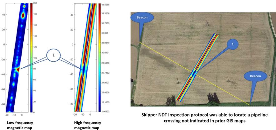
**Figure 6.** On the left side, high frequency and low frequency magnetic maps showing an anomaly tagged with (1). These anomalies illustrate the presence of a pipeline crossing the inspection area horizontally. On the right side, the position of the anomaly is correlated to the true position of the crossing pipeline.
